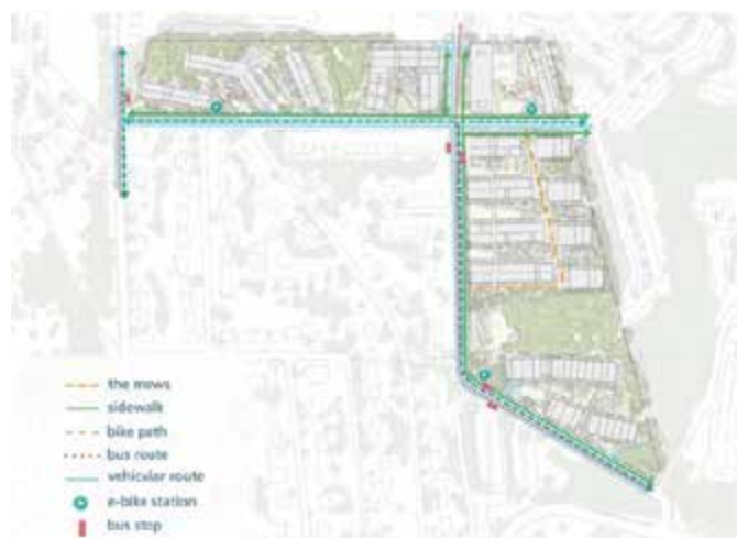
Figure 32: Streets and Sidewalks
